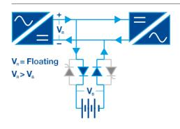
Battery is charged controlling the dynamic battery switch diodes on an intermittent basis, as per battery manufacturers recommendations, or after a discharge has occurred.
