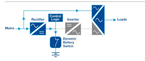
Ultra High Efficiency interactive mode: if input mains stability and reliability is outside preset limits, Ultra High Efficiency interactive mode of operation is activated. Loads are fed by the mains and the inverter is turned on and off by the control logic to stabilize UPS output and the rectifier keeps full battery capacity. That's what we call Very High Efficiency (VHE) mode. Efficiency is 97%, due to the transient inverter and rectifier contribution to overall losses.
